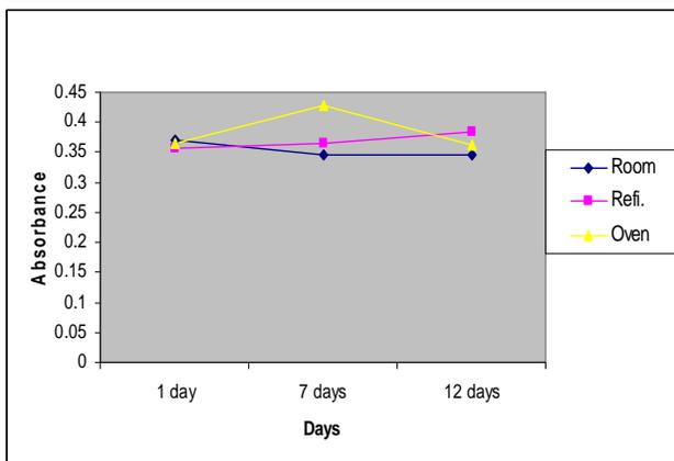
Fig.8 - Absorbance of coconut sugar syrup when stored under different conditions of room, refrigerator and oven for 7 and 12 days.
