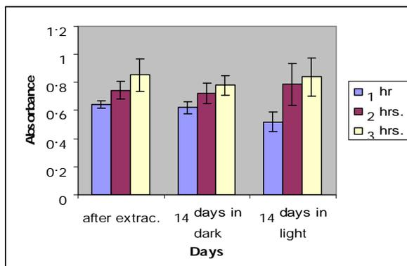
Fig. 4 - Graph comparing absorbance of extracts at 50°C when stored in light and dark room for 14 days
